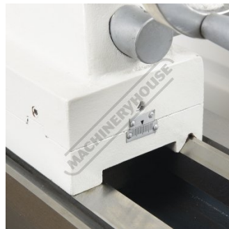
Tailstock Horizontal Adjustment
