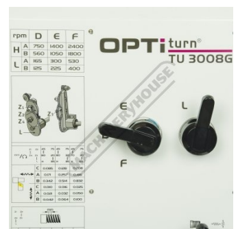
Spindle Speed Levers and Speed Chart
