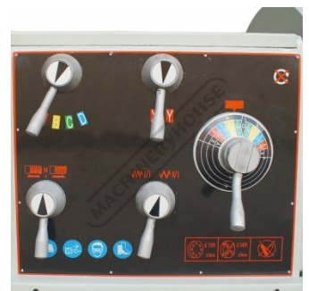
Spindle Speed Controls
