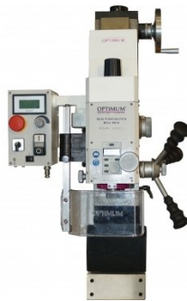
M647 Opti-Mill Head Attachment - Geared & Tilting Head
