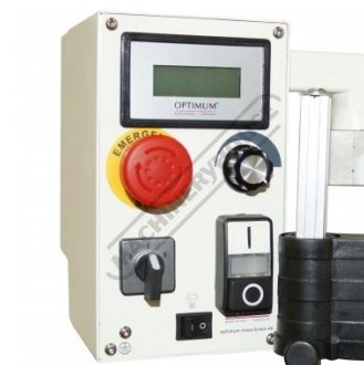
Variable Spindle Speed & Spindle DRO
