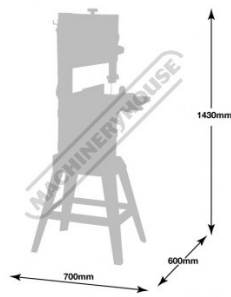
Minimum Floor Space Required
