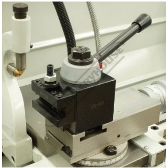
Quick Change Toolpost with 4 Holders
