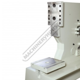
Solid Punching Base With T-Slot Grooves
