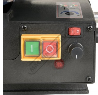
On Off Switch & Variable Blade Speed Dial
