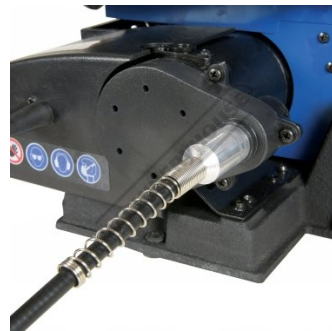
Drive Connector For Flexible Shaft Attachment
