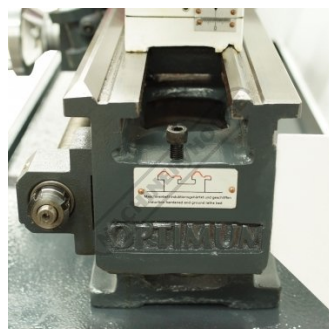
Induction Hardened and Ground Bed
