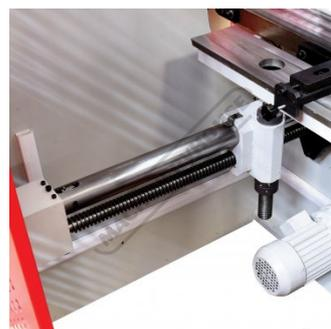
Estun NC E21 Control Ballscrew Backgauge
