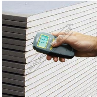
Measuring Moisture Content in Building Materials
