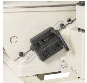
In-Feed Table Height Stop Setting
