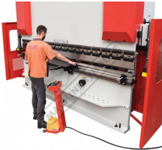
Laser Guarding system In Use
