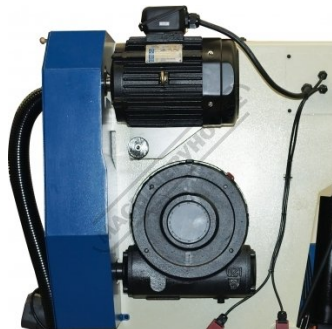
Industrial Motor and Gearbox Drive
