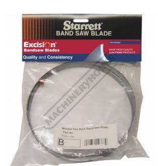
\$210.00 \$231.00 ORDER CODE: B601 Suits Band Saw Models: H-460HA-NC Blade Size (L x W x T) (mm): 5440 x 41 x 1.3 Number of teeth per inch (TPI): 3-4 Blade Type: BI-METAL Blade Suitable for - Material Type: Mild & Stainless Steel Suits Section Size (mm): 81-120
