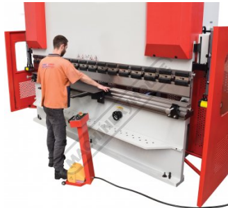
Laser Guarding system In Use
