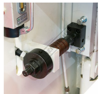
Quick Action Blade Clearance Adjustment
