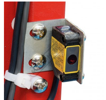
Safety Omron E3ZS Rear Light Sensor Guarding
