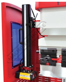
Laser Guarding System with Alignment Guide
