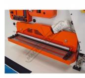
Optional Hydraulic Holddown for Flat Shear Optional Pipe Notcher
