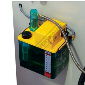
Auto Lubrication System
