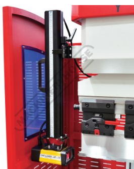
Laser Guarding System with Alignment Guide
