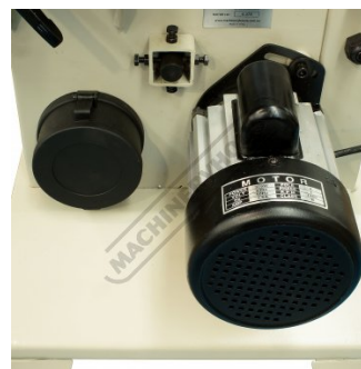
100mm Dust Port and Motor
