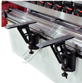
Adjustable Sliding Front Sheet Supports
