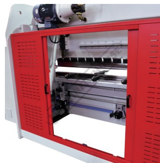
Servo X-R Axis Back Gauge
