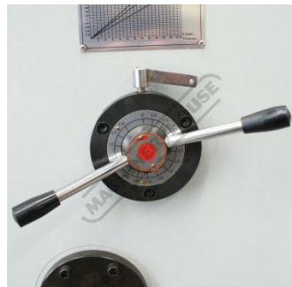
Rapid blade clearance adjustment
