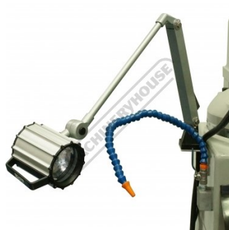
Halogen Worklight and Coolant Hose
