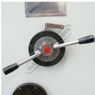
Rapid blade clearance adjustment
