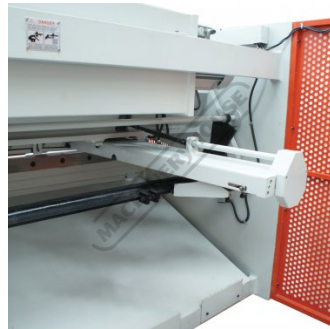
1000mm Powered ballscrew back gauge
