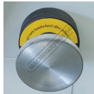
Fine Adjustment Dial for Backgauge
