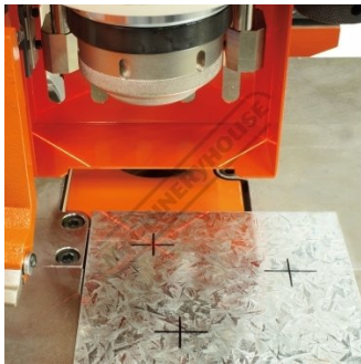
Laser Line On Galvanised Steel
