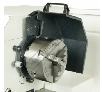
Safety Chuck Guard Open Position
