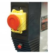
Emergency Stop Switch and Light Switch Work Light
