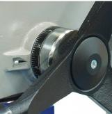
Drilling Depth Stop Setting With Scale
