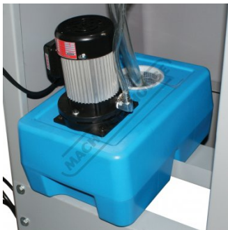
Coolant Pump and Tank
