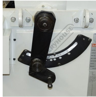
Rapid Blade Adjustment for Material Thickness
