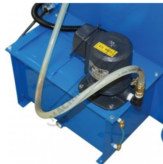
Coolant Pump and Tank
