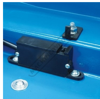
Safety Micro Switch on Pulley Guard
