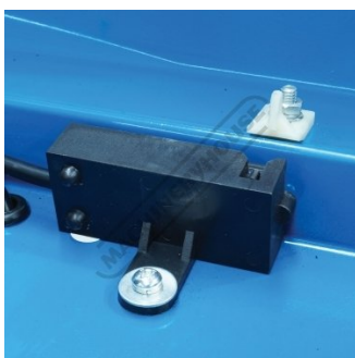
Safety Micro Switch on Pulley Guard
