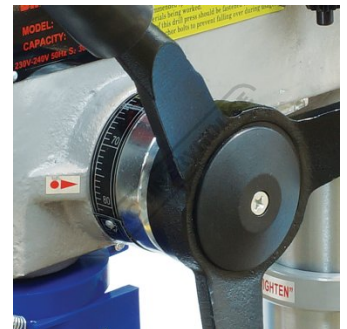
Drilling Depth Stop Setting With Scale
