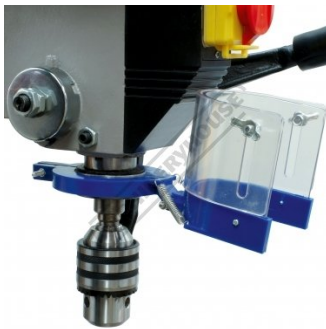
Safety Chuck Guard Flipped Up
