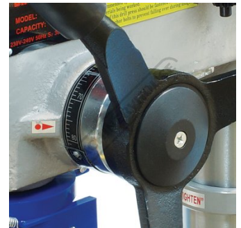
Drilling Depth Stop Setting With Scale
