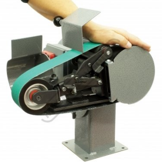
Depressing Belt Tensioner
