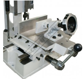
Dovetail Slideways on Work Table
