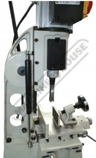
Gas Strut to Counterbalance Head Weight
