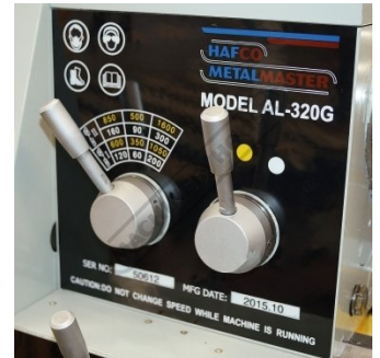
Spindle Speed Level Selectors 12 Speeds 16 1600RPM
