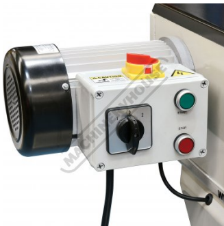
2 Speed Motor and On Off Switch
