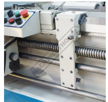
Leadscrew and Feedscrew Support Recovered
