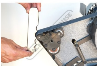
Small Wheel Selection for Notching & Contouring
