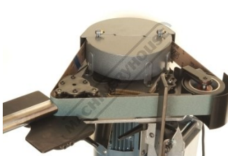
Tilting Table for Contouring & Pipe Notching
