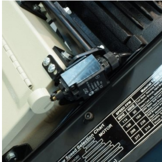
Blade Guard Safety Micro Switch on Right Side
