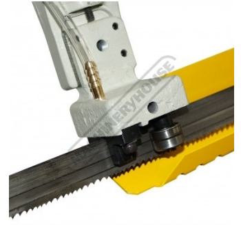
Carbide Blade Guides With Bearings
