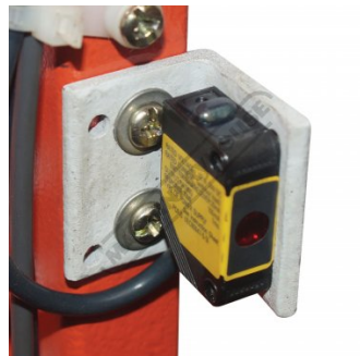
Safety Omron E3ZS Rear Light Sensor Guarding
