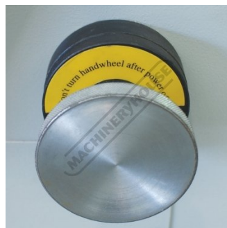
Fine Adjustment Dial for Backgauge
