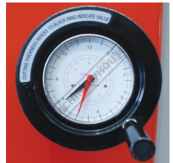
Variable Blade Gap Adjustment Dial
