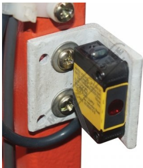
Safety Omron E3ZS Rear Light Sensor Guarding
