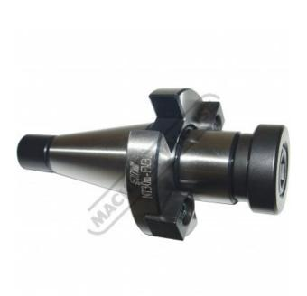
\$60.00 \$66.00 ORDER CODE: M542 MODEL: NT30 - FMB27-20 Draw Bar (mm / inch): 12mm D (mm): 27 H (mm): 20 K (mm): 7 54 C (mm): L (mm): 20
