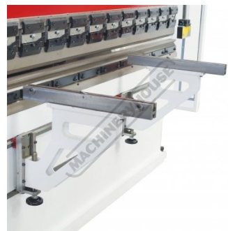
Sliding Front Sheet Supports on Linear Guideways
