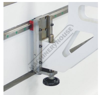
Front Sheet Support Height Adjustment
