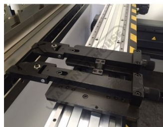
Servo driven Universal Backgauge Fingers
