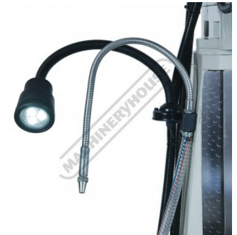
Work Light and Coolant Hose
