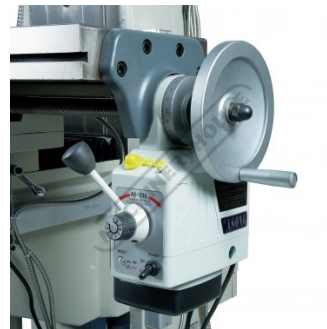
X Axis Power Feed with Rapid
